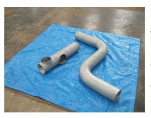
pipes for ship rigging. Pipe bending work is normally done by welding pipes to joints. Sunlight, however, does its bending work without cutting or heating pipes, but rather through a proprietary cold pipe bending process to create seamless, joint-free pipes. In addition, a T-piece is normally used to open many holes in a single pipe, but Sunlight has
